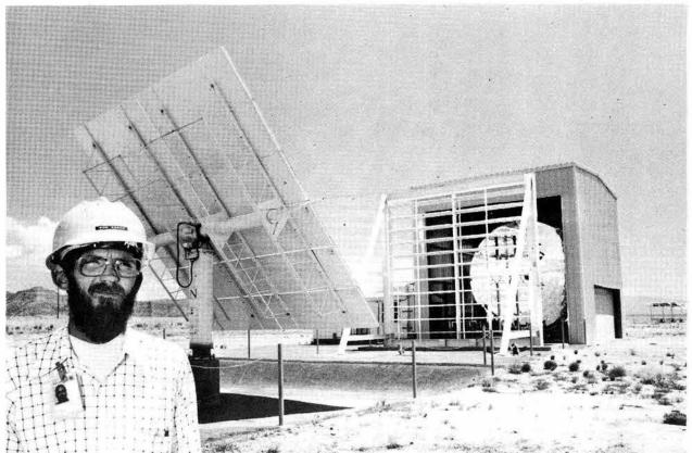
The heliostat reflects sunlight through the attenuator, a slatted device like a venetian blind that controls the power level and flux density. When the slats are open, the sunlight strikes 228 focusing mirrors arranged in a parabolic dish 22 feet in diameter.
